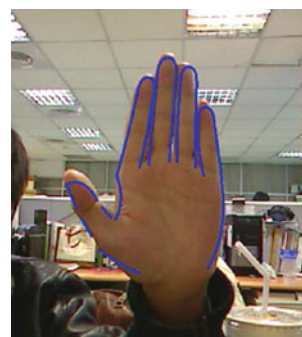
Fig. 5 The hand contour after applying the edge detection
