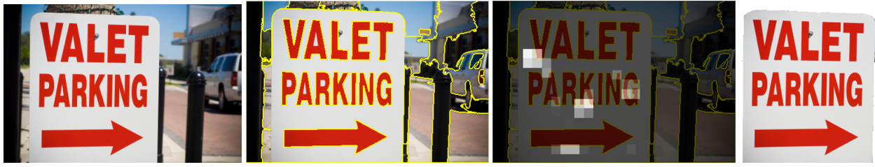
Figure 4. Saliency Based Region Extraction. From left to right: Original image, segmented image, segmented image with a gray scale importance superimposed on it, extracted image region.
