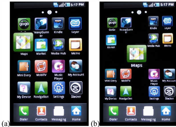
Figure 3. Example of a user interface adaptation : highlighting the maps icon by (a) increasing its size relative to other icons and (b) positioning the icon at the centre of the screen and decreasing the relative size of other icons. In this case the user is expected to use the maps icon next as per the prediction of the model
